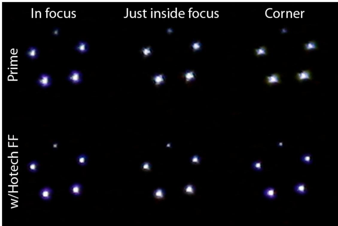
*Figure 2: Single frames from an artificial star test (Hubble Optics 5-star artificial star) taken at best focus in the center of the frame (left), just inside this focus point (middle) and at best focus but from the corner of an APS-sized frame (right). Individual frames were taken both at prime focus (top) and with the addition of a Hotech SCA Field Flattener (bottom). The slight deviations from round here are the result of thermal effects ("local seeing" effects) and not a cause for concern.*
